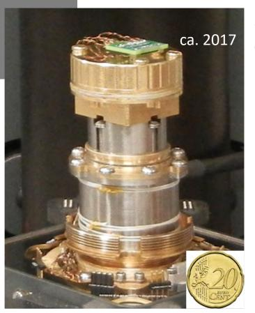
Carbon nanotube radiometer Shipping to CENAM in 2017 for intercomparison
