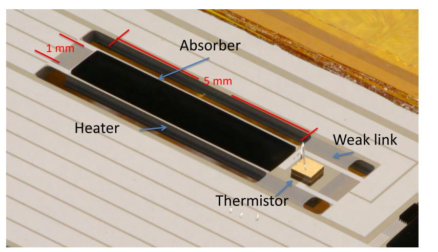
Carbon nanotube absolute radiometer
