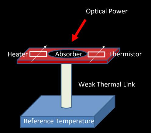
Optical Power Traceable to the SI by Electrical Measurements resistance, current, voltage
